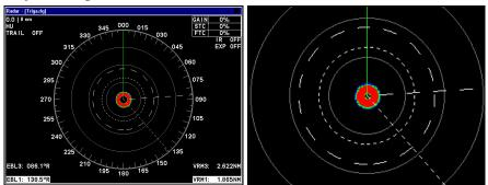
Increase Trigger Delay to diminish the size of the red ring (left). To set Trigger Delay correctly, reduce the ring to as small a size as possible, while keeping a black circle in the middle (enlarged view, right).
